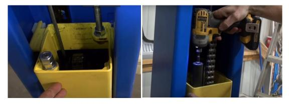
Congratulations, you're almost done. Now it's time to set a car on the lift, raise it just slightly off the ground, check it for balance, and again re-adjust your cables to ensure the vehicle is level from side to side. Now you're done, but we do recommend checking your anchors again after a month or so of usage to make sure any initial loosening of the anchors isn't allowed to remain. We hope this was helpful! Please check us out at <u>www.RedlineStands.com</u> to see all the lifts we offer.
